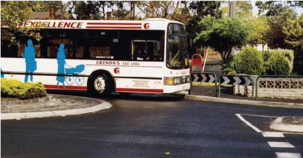
Figure 5.4.6.2: Front overhang on low-floor bus. Source: Austroads Guide to Road Design Part 4B Roundabouts
