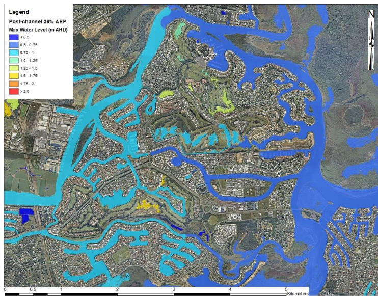
Figure 15. Maximum Floodwater Height - 39% AEP Post-channel
