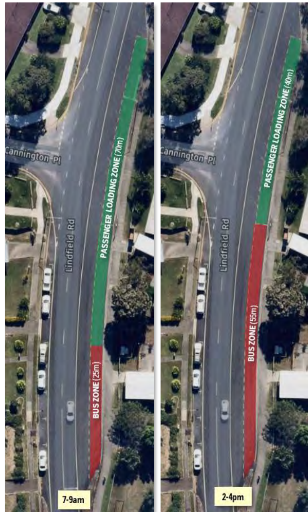
FIGURE 4: Passenger loading zone arrangements – AM and PM school days Source: Nearmap (image taken 7/6/22)
